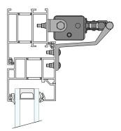
Projected top-hung, parallel opening window, outward opening
