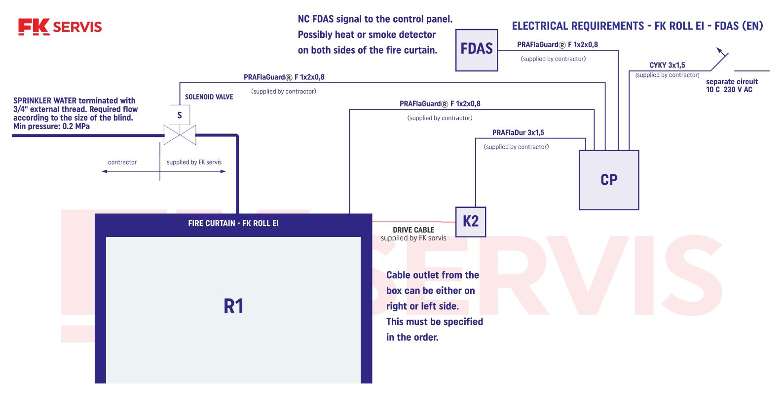
CP: control panel FK ROLL +, 400x300x150 mm, surface mounting, steel box, cable inlet ot top side
